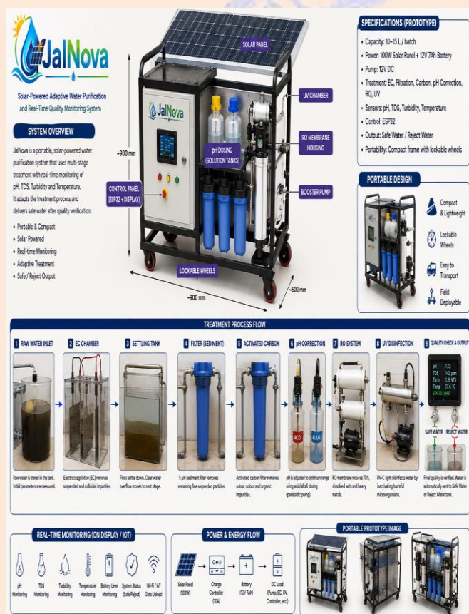
Figure 1. Proposed JalNova prototype and treatment architecture (concept illustration from the project report).
