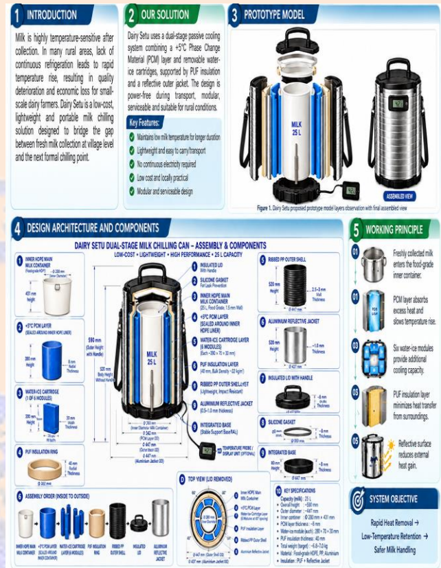
Figure 2. Integrated Dairy Setu infographic: prototype model, component architecture, assembly details and working principle.
