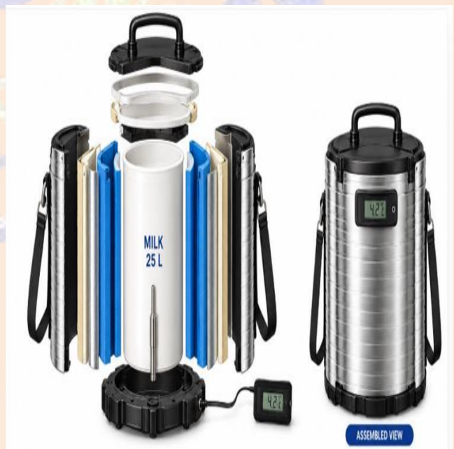
Figure 3. Exploded and assembled views of the proposed Dairy Setu milk-chilling can.
