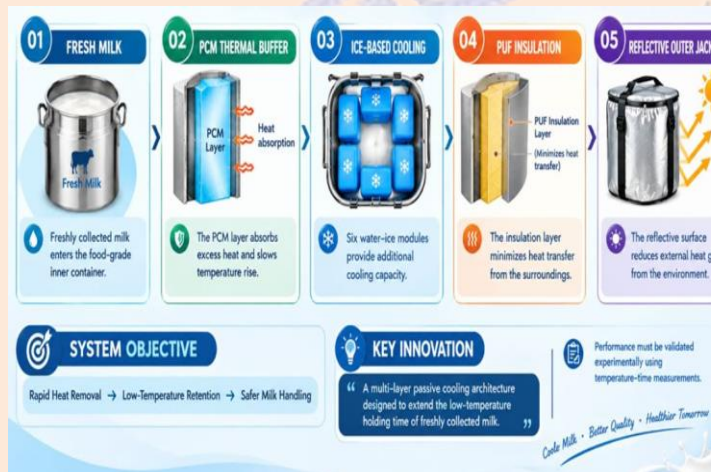
Figure 5. Conceptual working sequence: PCM thermal buffer, ice-based cooling, PUF insulation and reflective outer jacket.
