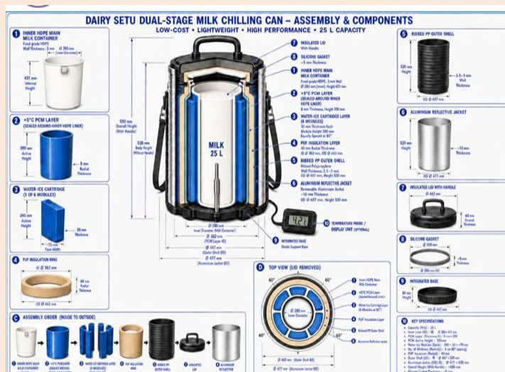
Figure 4. Technical assembly drawing and component specifications of the proposed 25 L system.
